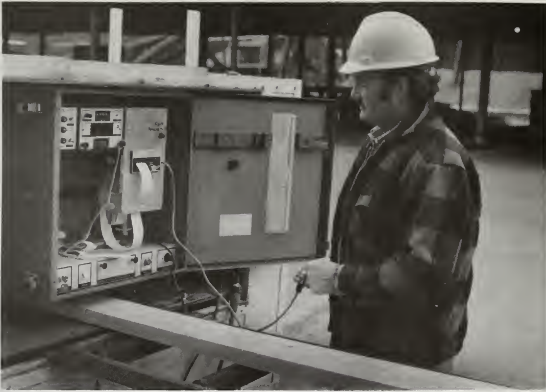
Calibration of a continuous lumber testing machine is an important aspect of overall quality control. This MSR machine separates high strength material for use in engineered wood structures (i.e., trusses, laminated beams).
